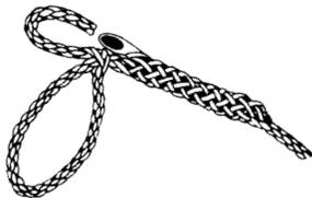
3. Just below the point where rope comes through, (Arrow) insert fid into rope in direction away from loop, as illustrated. Insert short rope end into fid and guide fid down the hollow center of the rope. Push fid forward with right hand . . . at the same time use left hand to work rope over fid.
